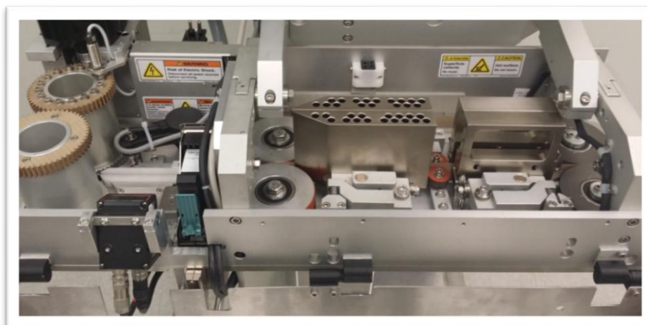
Validatable Sealing Head with Datamatrix Printer & Keyence Code Reader
