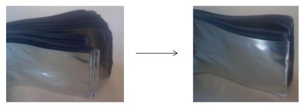
Make sure all pouches are facing the same way and that they are loaded into the magazine as neat as possible. When the magazine is completely empty, it is recommended to carefully place 2 or 3 pouches in position to create a good base, then load small stacks of about 20 pouches on top of those. The total number of pouches that a magazine can successfully hold is dependent on pouch size, configuration, and stability.
